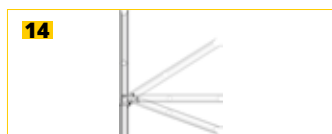
14 Folding upright H : 1010 - aluminium joint WV8201010F
