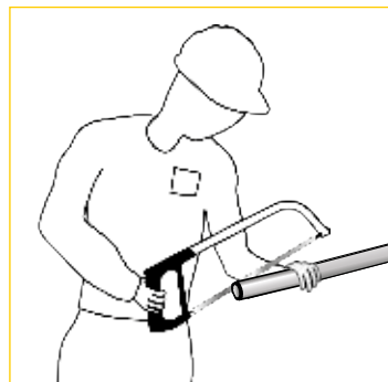
16 - Adjust last section by sawing swagged extra
